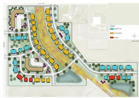
areas, and is colored coded by construction type (walkout basement (red), basement (teal), and or no basement (mustard)).
