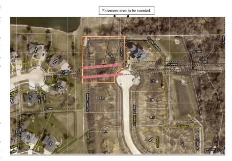
from 60 feet to 40 feet wide by vacating a 10-foot portion of the existing 60-foot sanitary sewer easement on the north and south sides of the existing easement. The owner would like to reduce the encumbrance on his lot so he can more easily develop the property.
